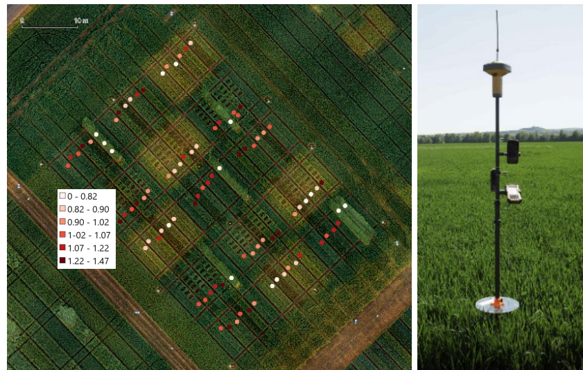
Fig. 1: Left: RGB orthoimage acquired with a DJI Phantom 4 UAV of the study site with the locations of the manual plant height measurements. Right: RTK GPS Laser Distance Winter Wheat Plant Height Measurer
